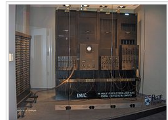
Four ENIAC panels and one of its three function tables, on display at the School of Engineering and Applied Science at the University of Pennsylvania
